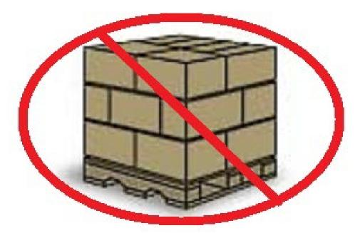
Carton overhang off the pallet can reduce stacking strength by up 32%.
