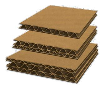
Also available, but not listed in the provided table, are multiwall corrugated boards containing four or more fluted mediums. These multiwall boards are used to manufacture heavy duty cartons such as may be required for bulk loads of raw castings or other heavy weight production materials.
